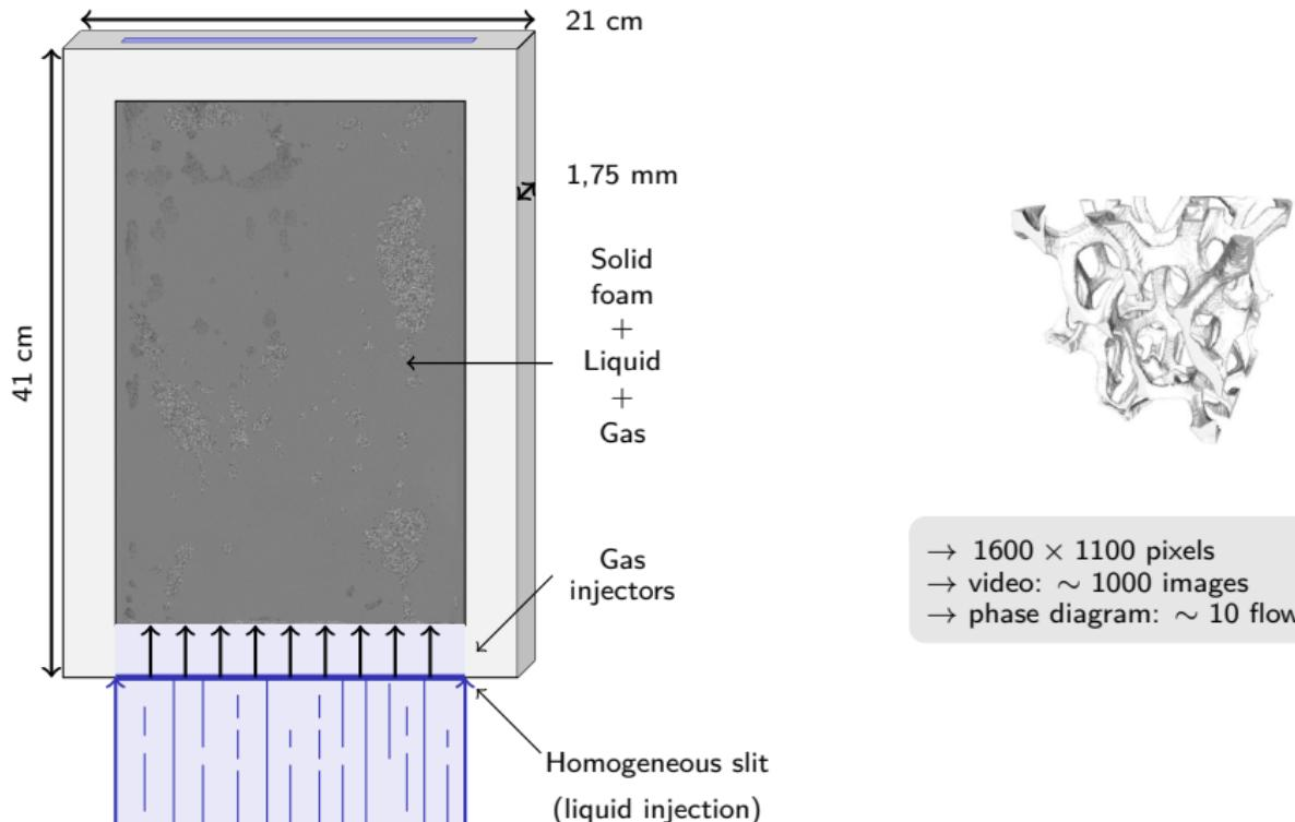
Low activity:  $Q_G = 300\text{mL/min}$  -  $Q_L = 300\text{mL/min}$
