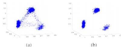
Fig. 2. Scatterplot of features in subspace. (a) Scatterplot of features projected onto the 3-d subspace. (b) Scatterplot after removing features with high edgehood.
